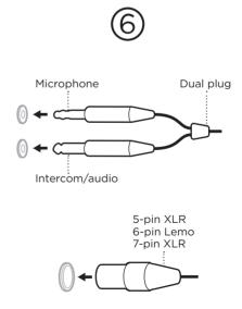
Insert the aircraft connector into the aircraft control panel.
