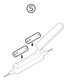
Insert the AA batteries (2) into the control module.
