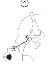
Grasp the microphone base, and adjust the boom so the microphone is 0.5" (12.7 mm) from your lips and the white surface on the base is facing your mouth.
