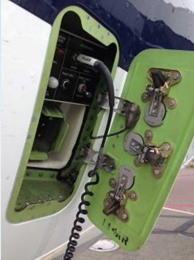
Interface Cord Flexed at 90 Degree Bend at Aircraft Connection
