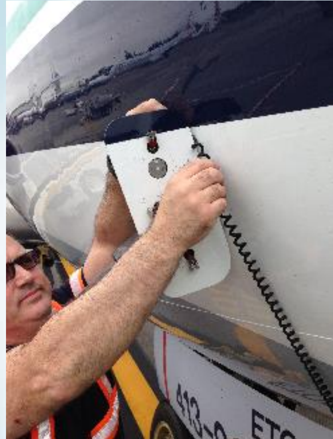
Interface Cord Pinched in Service Panel Door
